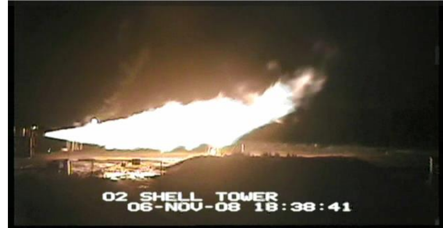
Test4. Scale: 10.4 pixels/m 50mm H2 Release
