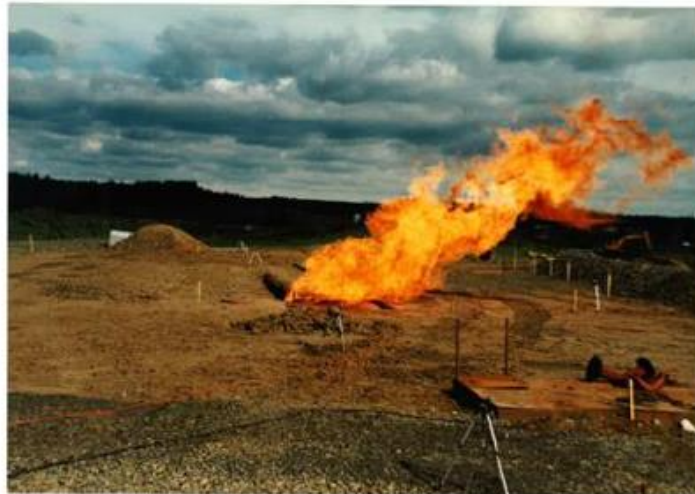
Experiment 8, NG, 75 mm, 0.5 bar, impacting
